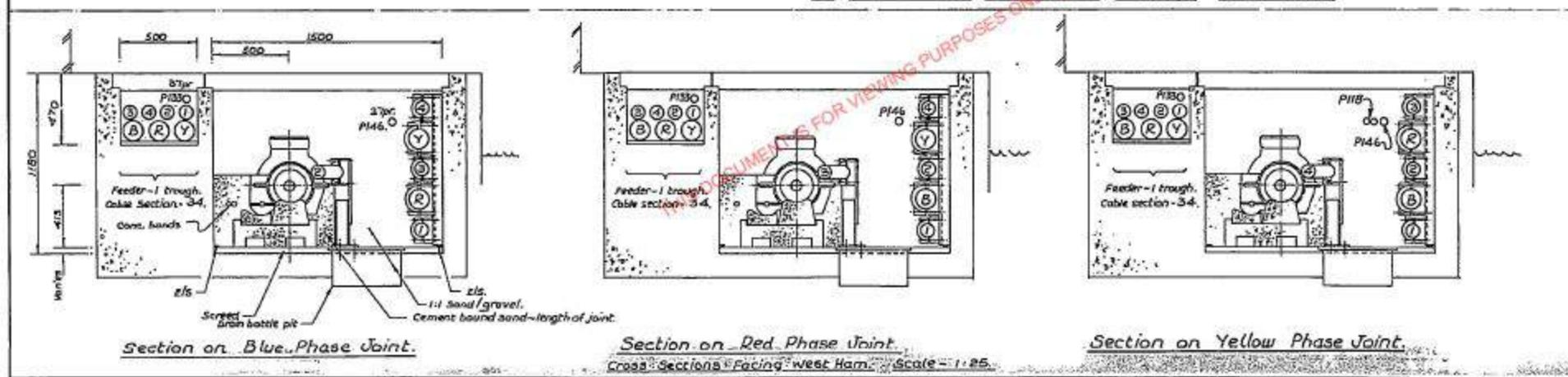
**Jointing Details ~ Feeder Cables.**
